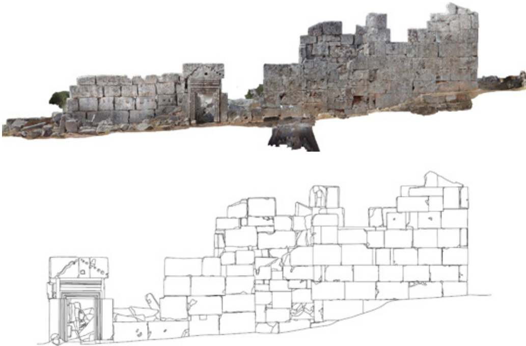
Fig. 8 Upper: Orthophotograph from top view. Lower: Top plan from the orthophotograph
